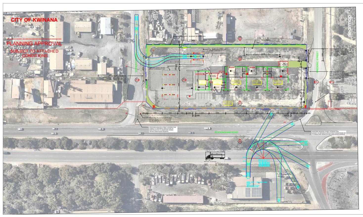
Proposed Service Station, Rockingham Road, Naval Base Main Roads WA: 19.0m Semi-Trailer - 15m Radius Fuel Tanker Entry LEGEND
